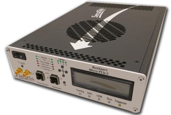
Figure 1: The BusXpert Micro 2 PCIe/NVMe Analyzer measures 7 inches x 10 inches x 2
