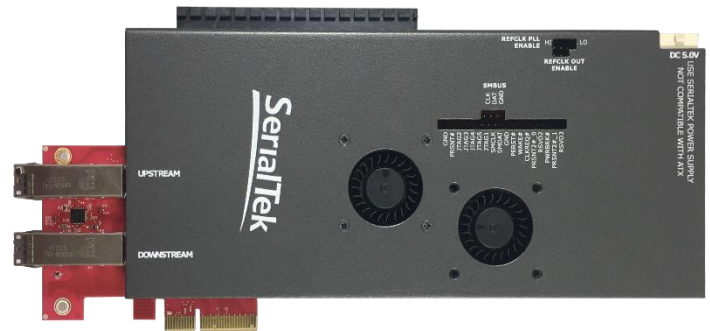
Figure 1: PCIe Gen3 x4, x8 Slot/AIC Interposer.
